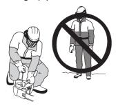
Always hold the saw with both hands. The right hand should be on the rear handle, and the left hand on the front handle. All people, whether right or left handed, should use this grip. Use a firm grip with thumbs and fingers encircling the chain saw handles.
